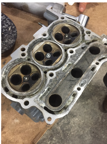
Engine part with mineral deposit build up.
